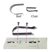
If using mounting brackets, line up the 2 small holes on the bracket with the 2 small holes on the back of the monitor and insert the 2 screws provided.
